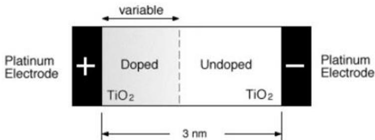
**Fig. 1.** Structure of a Physical Memristor [8]
