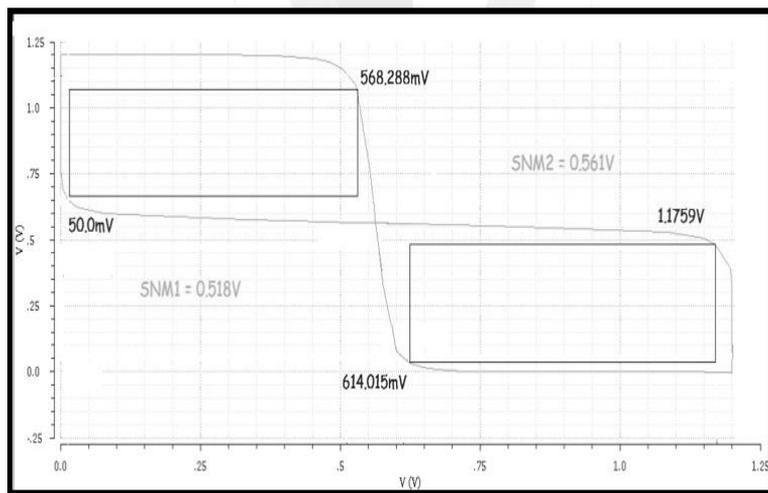
**Fig. 11.** Hysteresis curve of proposed 7T1M-NVSRAM cell
