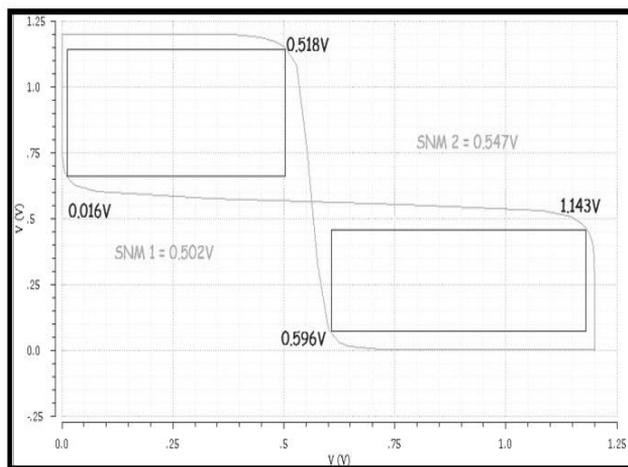
**Fig. 8.** Hysteresis curve of 6T SRAM
