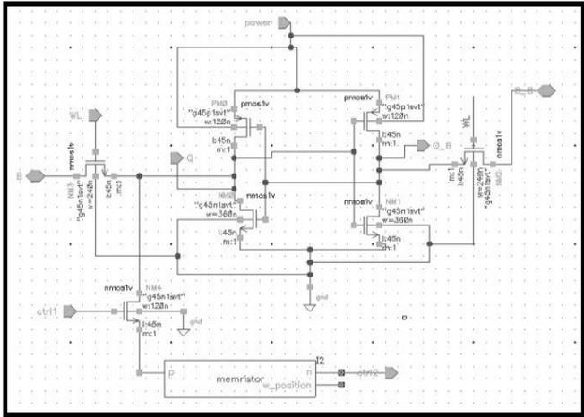
**Fig. 4.** Circuit structure of proposed 7T1M-NVSRAM cell
