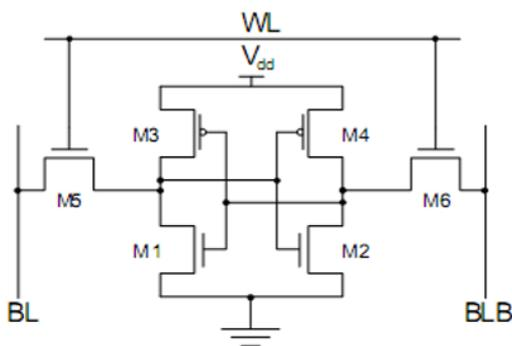
**Fig. 2.** Schematic of Conventional 6T SRAM circuit
