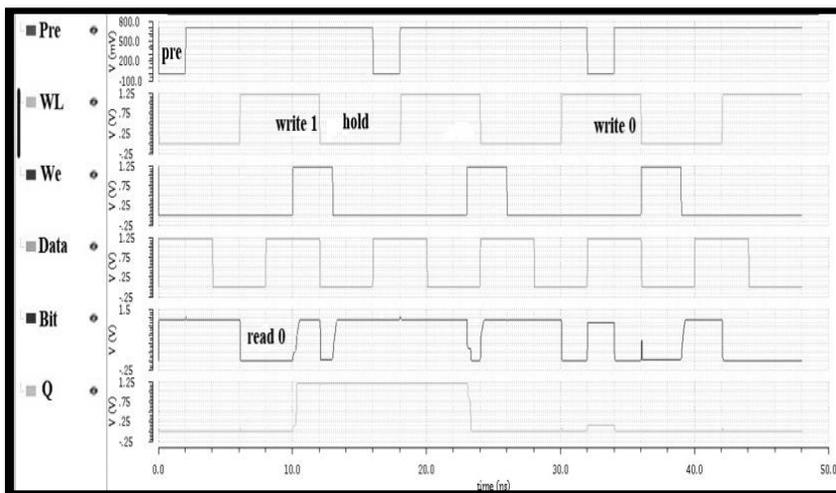
**Fig. 7.** Read and write operations of a 6T SRAM
