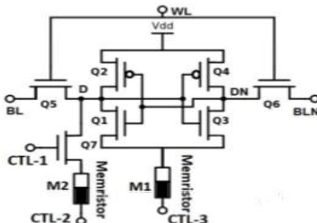
Fig. 3. Circuit structure of 7T2M- NVSRAM cell [5]
