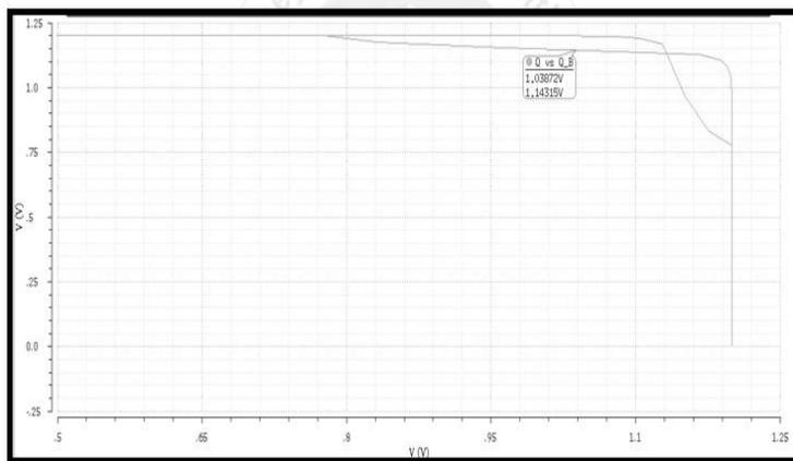
**Fig. 9.** Hysteresis curve of a 7T2M-NVSRAM cell
