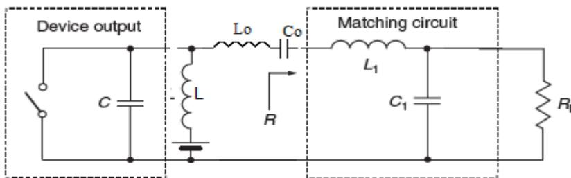
**Fig. 1.** Equivalent circuit of Reactance compensation network [1]
