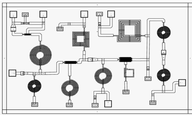
**Fig. 7.** Layout of Class -E Power amplifier with linear-mode pHEMT linearizer circuit.
