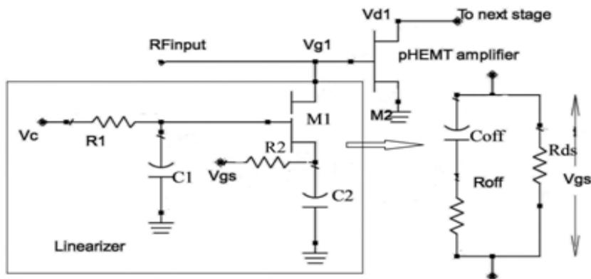
Fig. 2. Linearizer circuit using pHEMT
