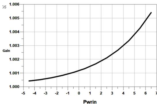
Fig. 3. Gain expansion with respect to Input power
