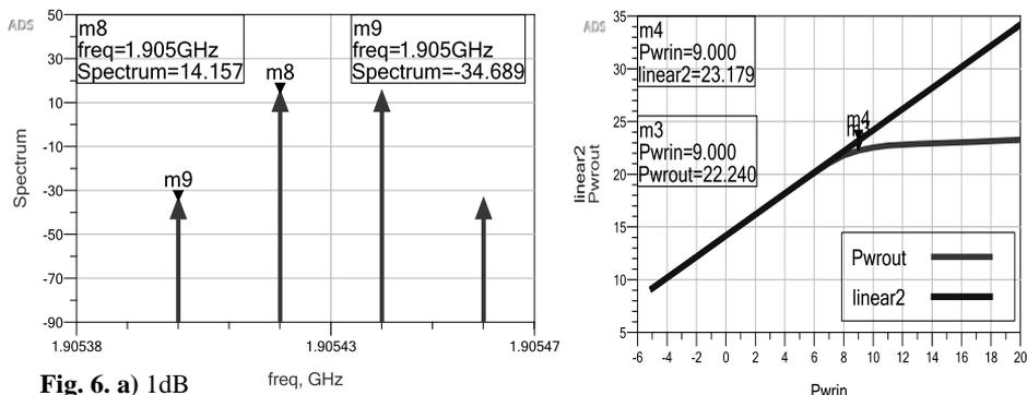
**Fig. 6. a)** 1dB compression point of Class-E PA with built-in Linearizer and **b)** Two-tone spectrum
