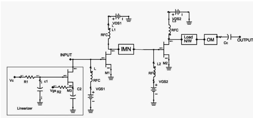
**Fig. 5.** Class E Power amplifier with pHEMT linearizer circuit
