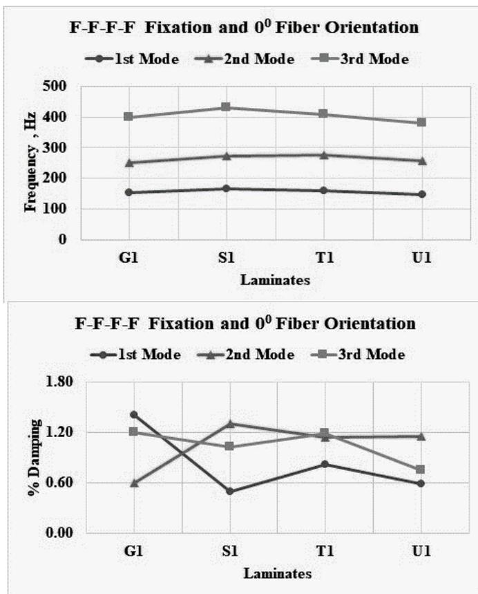
Fig. 4. a) Natural frequencies in F-F-F-F fixation and b) Damping (%) in F-F-F-F fixation
