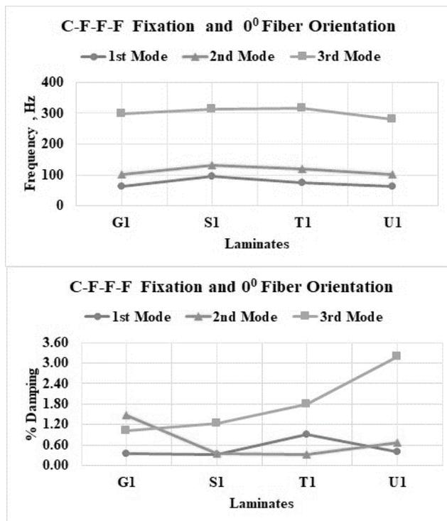
**Fig. 5.** a) Frequency for C-F-F-F fixation and b) Damping for C-F-F-F fixation
