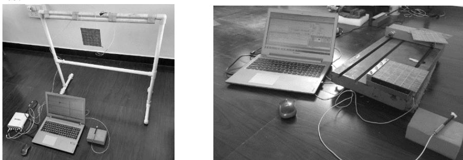
Fig. 3. a) Experimental setup for F-F-F-F fixation and b) Experimental setup for C-F-F-F boundary condition
