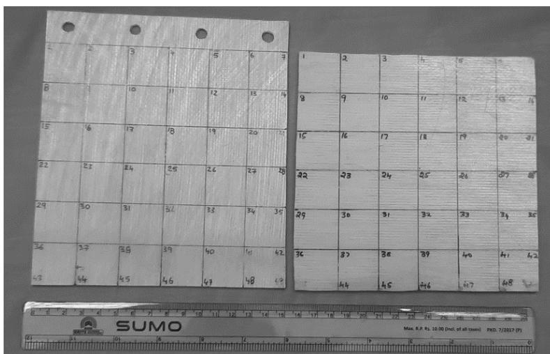
Fig. 2. Specimens with 1- 49 grid points for C-F-F-F and F-F-F-F fixations
