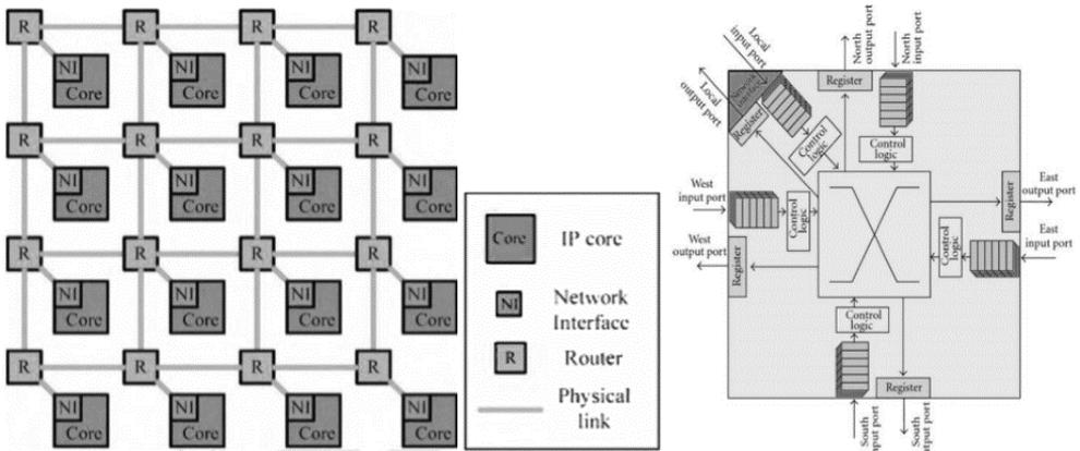
**Fig. 1. a)** Mesh based NoC architecture and **b)** Typical NoC router architecture [2]
