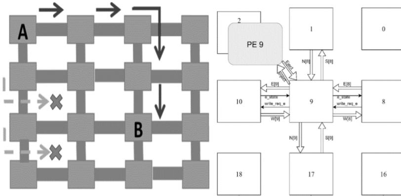
Fig. 2. a) Packet path from Source (S) to Destination (D) [4] & b) Schematic of process node [2]
