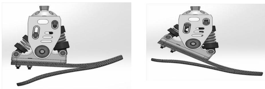
**Fig. 3.** Position of spring a) Dorsiflexion (toes closer to the shin) and b) Plantarflexion (toes away from shin)
