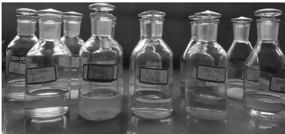
**Fig. 4.** Saturated salt solutions corresponding to different relative humidity
