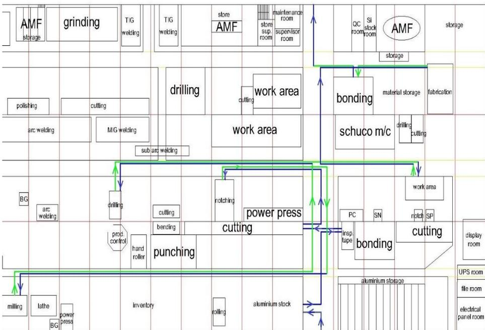
Fig. 5. Material flow process for aluminium panels
