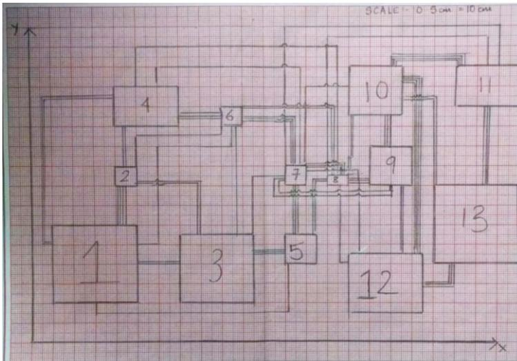
Fig. 7. Space Relationship Diagram - Al Fabrication
