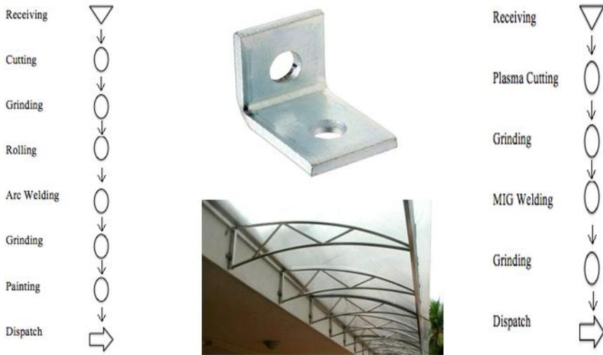
**Fig. 2.** Operation process charts for MS brackets and canopies
