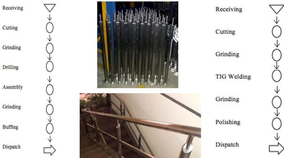
**Fig. 3.** Operation process charts for SS pipes and railings
